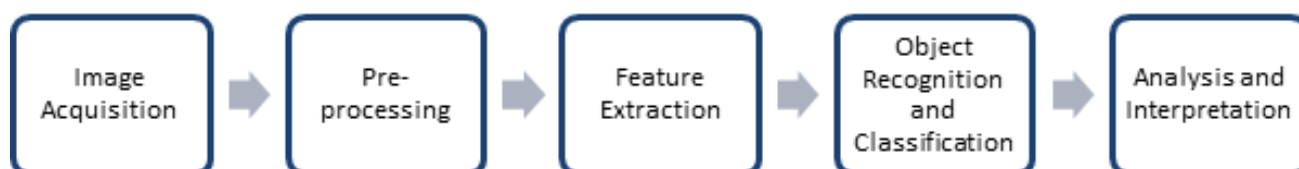
Fig 2. Steps in the Computer vision process
